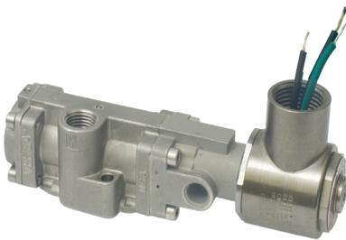
The Versa C316 Series stainless steel NAMUR valve 5-port design can be ordered as either a 4-way for double acting actuators, or as a 3-way for spring return actuators. When the 3-way function is utilized, the unused exhaust port becomes an actuator vent where a filter/muffler can be installed to prevent contaminants from entering either the valve or the
