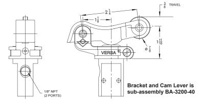
Actuated by cam movement in either direction. Cam follower is hardened.
