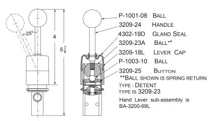
Light force, offsetting the handle 25° from vertical, is sufficient to operate
