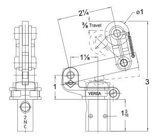
Bracket and Trip-Cam Lever is sub-assembly BA-3200-40-35.
